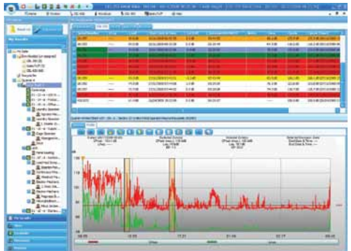
Tree style database of results with colour coding for exceeded noise action levels
